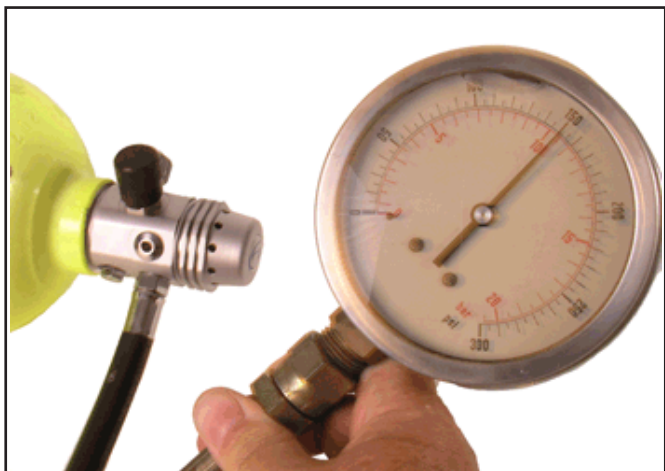
Checking the Intermediate Pressure with a Gauge
