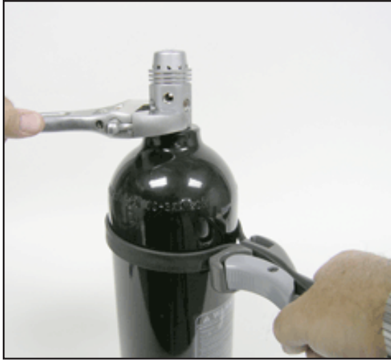
Removing the RaZor from the Cylinder
